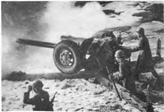
Figure 6-27. 122-mm howitzers. The M-30 (above) and D-30 (below) are the standard divisional artillery weapons in Soviet Ground Forces. The newer D-30 has a maximum range of over 15,000 meters.
